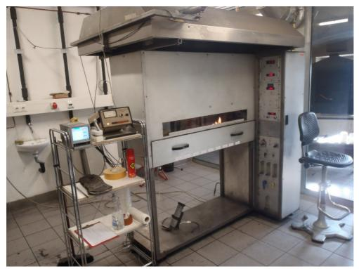
Radiant Panel Test, EN ISO 9239-1
