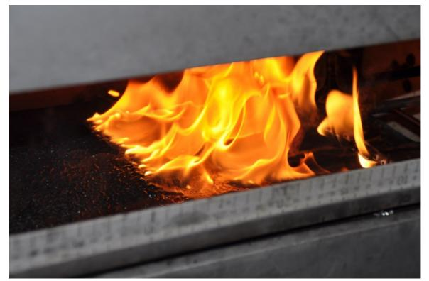
Radiant Panel Test, EN ISO 9239-1
