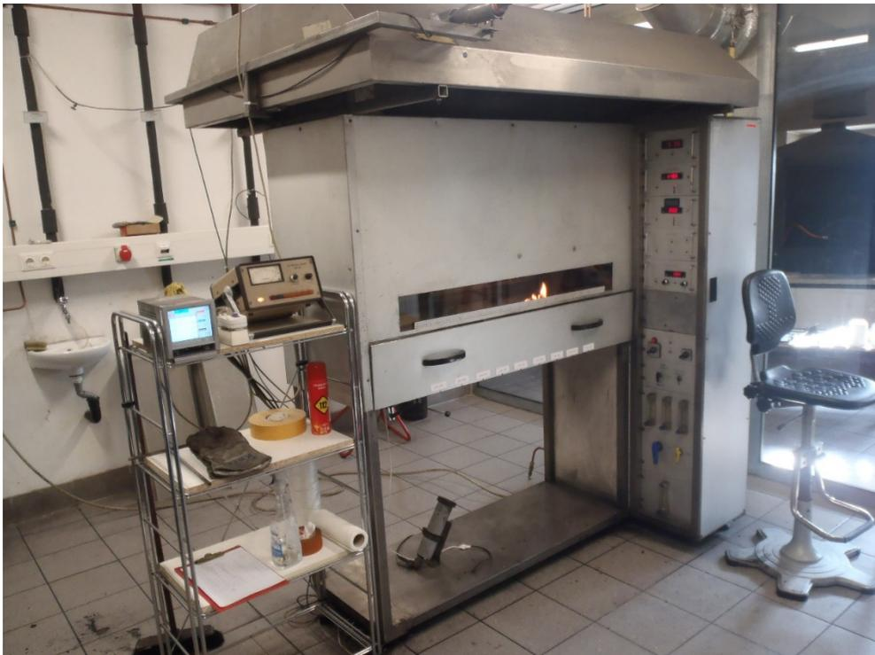
Radiant Panel Test, EN ISO 9239-1
