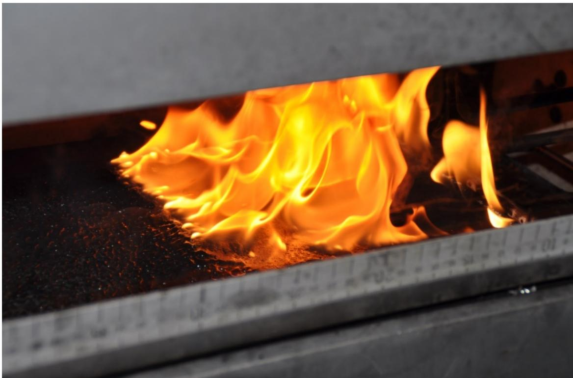
Radiant Panel Test, EN ISO 9239-1
